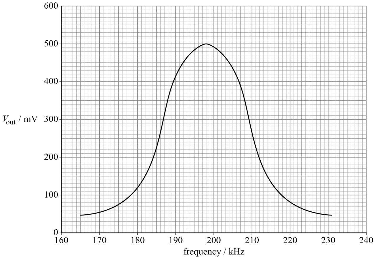
Determine the bandwidth of the filter circuit.
