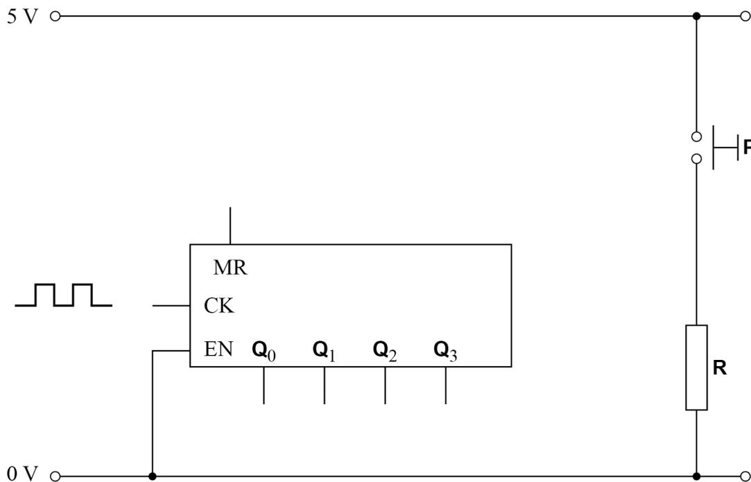
The counter resets when the master reset pin MR receives a logic 1
